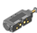
kontrolni ventil 5/2-kraki ventil co-ax, elektro-pneumatski, G1/ 4, p = 4 - 10bar
